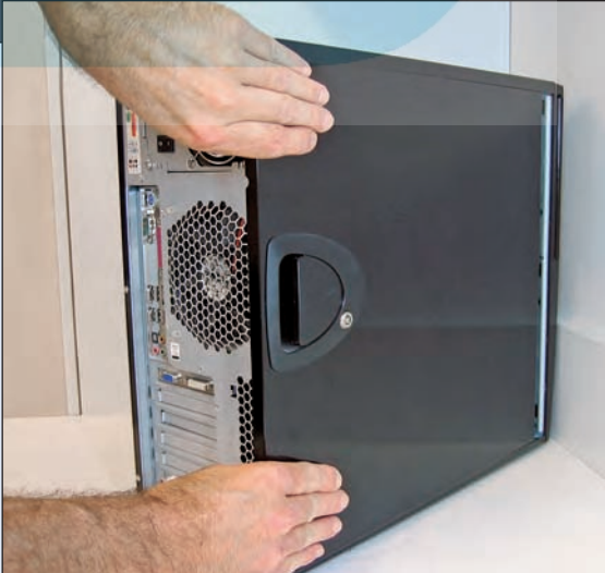
Color Plate 3: After removing the thumbscrews, slide the cover off by pulling it to the rear.
